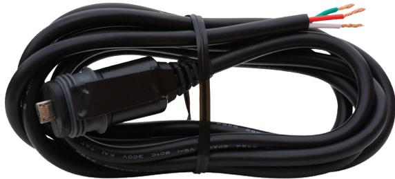
The external three-wire hardwire kit is used to hardwire into a vehicle's 12/24 VDC power system. Wiring can be done through center/rear brake light, or another external power source. Ensure the cable is properly grounded.
