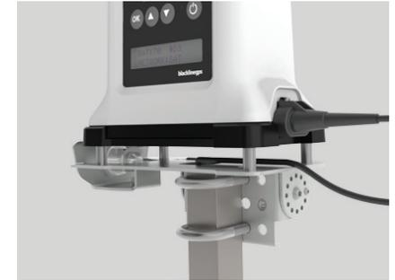
Screw the multi-purpose mount to the G7 Bridge Mounting Bracket plate. Attach the G7 Bridge Mounting Bracket to roof rack, bed rack or pole/post using the appropriate u-bracket size. Slide and snap G7 Bridge into the multi-purpose mount, and lock the G7 Bridge Mounting Bracket with key for additional security.
