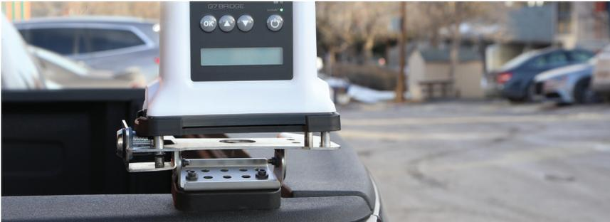
Screw the anchor point into the truck bed rail, and then attach the G7 Bridge Mounting Bracket to the anchor point using screws. Screw the multi-purpose mount to the G7 Bridge Mounting Bracket plate. Slide and snap G7 Bridge into the multi-purpose mount, and lock G7 Bridge Mounting Bracket with key for additional security.
