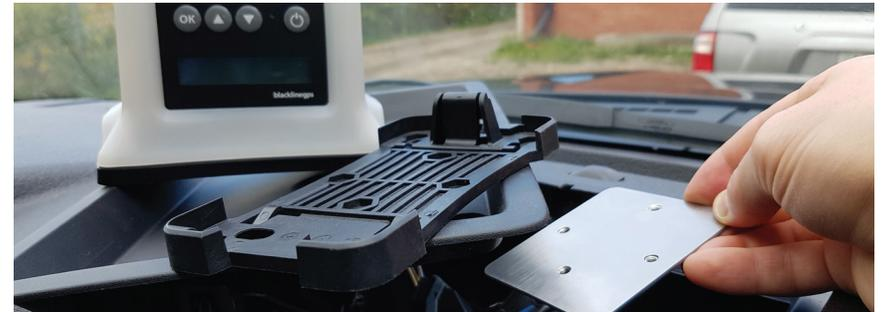
Remove the dash tray or portion of the dash you want to mount to. Screw the multi-purpose mount to the top of the dash, then screw the dash plate under the dash tray to secure the mount in place. This is best suited for a Ford F-150 with removable dash tray to avoid drilling directly into vehicle dashboard.
