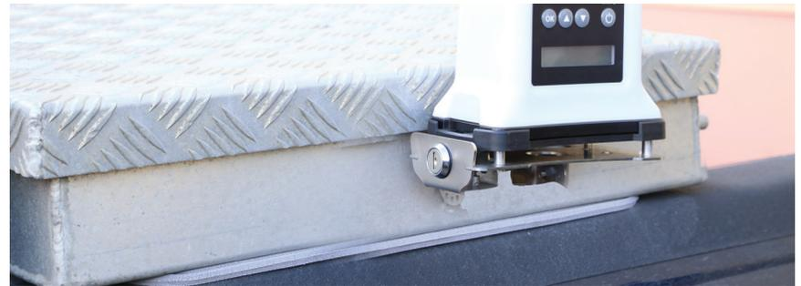
G7 Bridge can be mounted to a truck bed tool box if it has an unobstructed line of sight to the sky. Screw the multi-purpose mount to the G7 Bridge Mounting Bracket plate, and screw the plate to the side of the tool box. Slide and snap G7 Bridge into the multi-purpose mount, and lock G7 Bridge Mounting Bracket with key for additional security. Ensure the LCD screen is facing outwards for operation.
