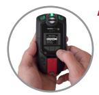
A: Use the up and down arrows to navigate to bump test or calibrate from the main menu
