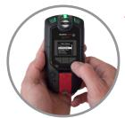
A: Use the up and down arrows to navigate to bump test or calibrate from gas options in the main menu
