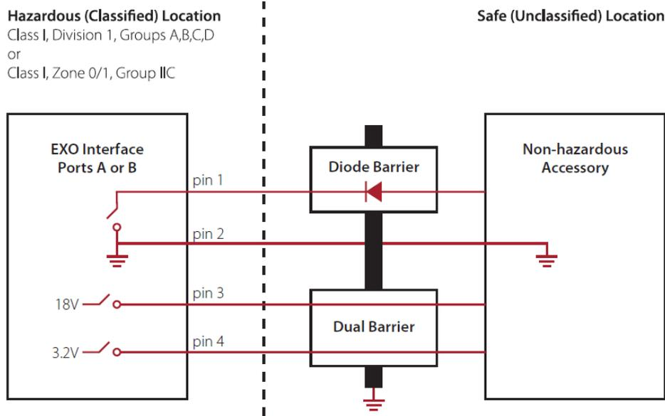
**NOTE:** A barrier is required for each interface port. The diode barrier and dual barrier can be individual units or a joint unit.
