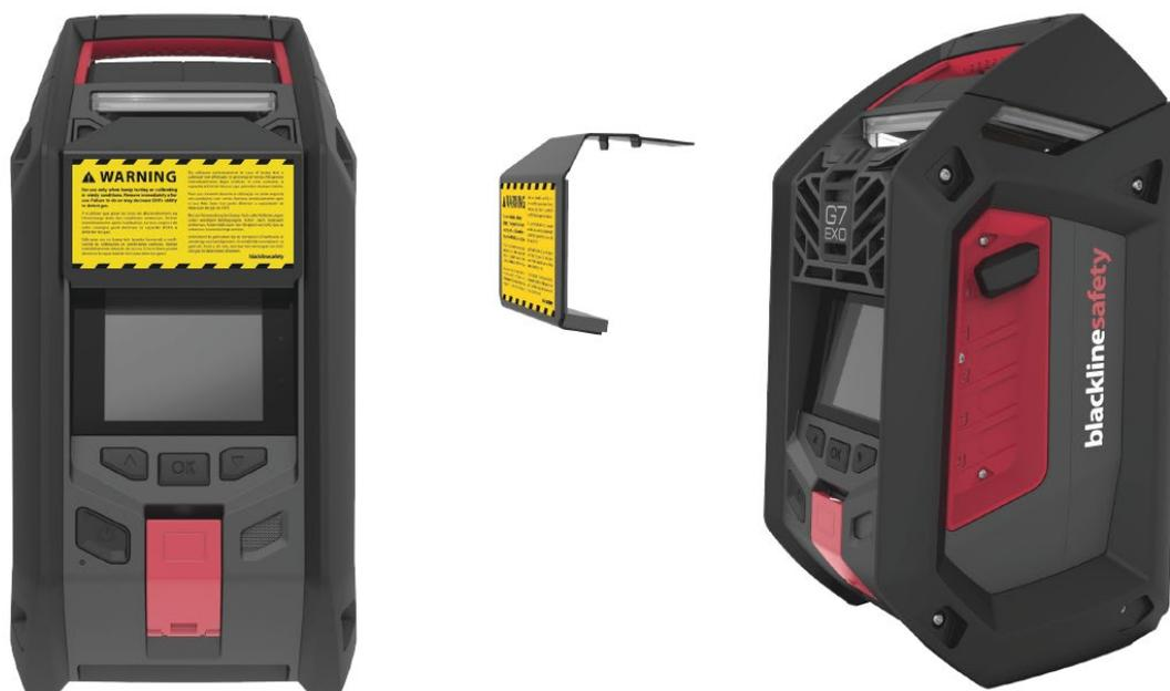
**▲ WARNING:** The Wind Guard MUST be removed when the bump test or calibration is complete. Failure to remove the Wind Guard will slow down EXO's response to hazardous gases.
