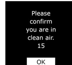
When powering on an EXO with an LEL-MPS sensor, the device will prompt you to acknowledge and approve that the device has been powered on in a clean air environment and a zero adjustment can take place. Should you fail to acknowledge the zero prompt within 15 seconds, your device will enter a latched alarm state and require that you power cycle the device and approve the zero prompt.
