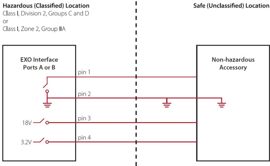
Functional output parameters for interface ports A and B - high output models
