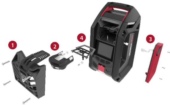
Figure 3-3: Uninstalling updated G7 EXO Diffusion components
