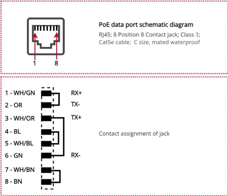
EXO Translator PoE data port aligns with the standard IEEE802.3af, power class 3 parameters:
