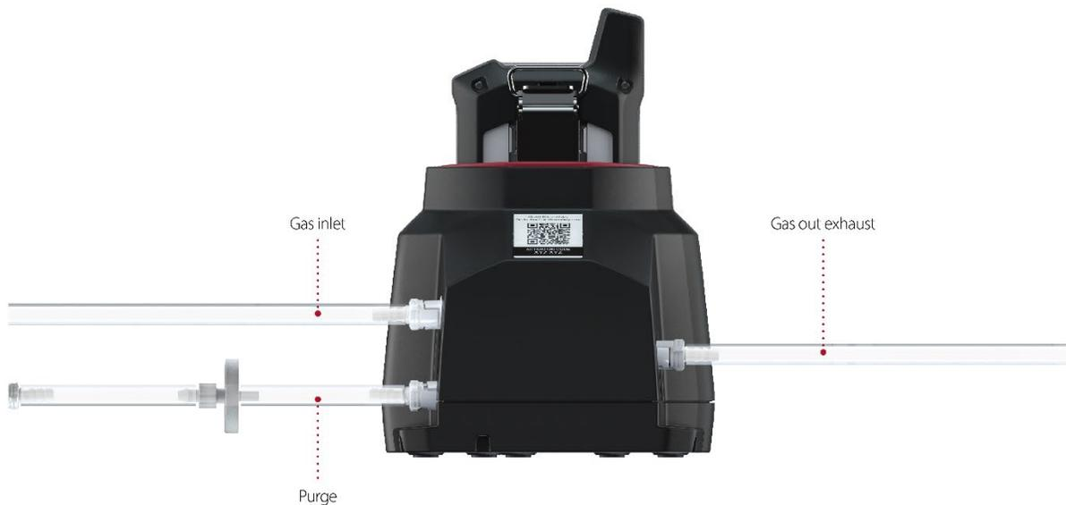
G6 Dock is equipped with Gas out exhaust, Purge gas inlet, and Gas inlet ports:
