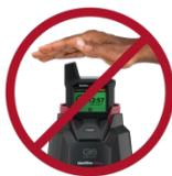
**IMPORTANT:** To ensure that the G6 and G6 Dock power and data contacts connect securely, avoid pressing G6 into the dock cradle using the antenna. Always lock G6 into the dock cradle by pressing directly down on G6's top indicator lights.
