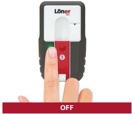
2. If you are updating a Loner Bridge, press the power button to turn it on and wait for the SureSafe™ green light to turn solid. If you are updating a Loner 900, press and hold the power button to turn it off.
